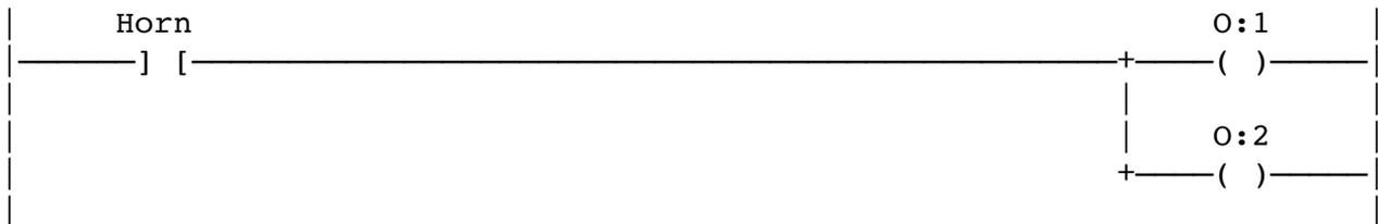
This rung will turn both output #1 and output #2 on when the Horn is operated.
